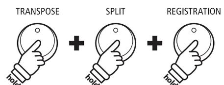
The piano will turn on in update mode, and the LED indicators for the three pressed buttons will start to flash.
