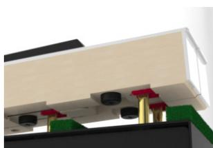
In addition to all new *Ebony Touch* key surfaces, the *Grand Feel II* keyboard action also features a revised hammer design, optimising the hammer's centre of gravity to improve the dynamic load of each key stroke. Counterweights are also attached to all 88 keys, and graded from bass to treble, ensuring consistent weighting across the length of the keyboard during both pianissimo and fortissimo passages.
