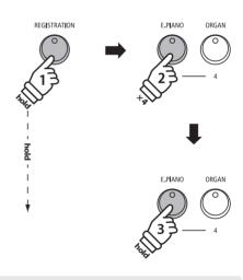
**Example:** To store the current instrument setup to memory 3D, press and hold the REGISTRATION button, press the E.PIANO button four times, then press and hold the same E.PIANO button.
