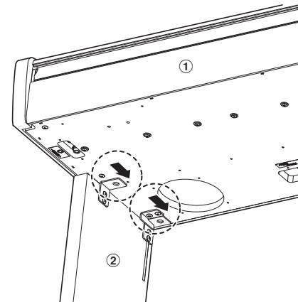
Secure the main body to the stand from below, using the four screws (with the flat washer and spring washer) ⑦.
