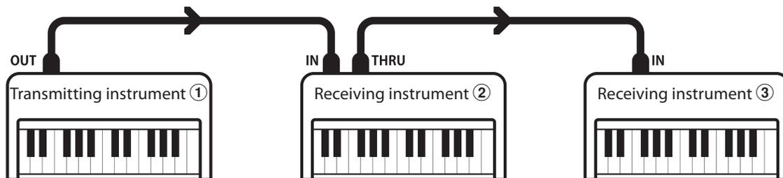
Transmitting instrument ① sends transmit channel and keyboard information to receiving instruments ②/③. The information arrives at the receiving instruments ②/③. Receiving instruments ②/③ will respond to MIDI data that is sent if their receive channel is the same as the transmit channel of the transmitting instrument ①. If the channels do not match, then the receiving instruments ②/③ will not respond to any data that is sent.
