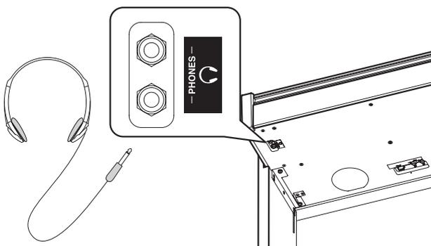
When a pair of headphones is connected, sound will not be produced by the speakers. Up to two pairs of headphones can be connected and used simultaneously.
