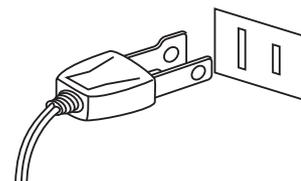
**This product shall be near the AC outlet and the power cord plug in a position so that it can readily be disconnected in an emergency because electricity is always charging while the plug is in the AC outlet even in a power switch off condition.**
