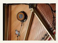
AURES instruments incorporate transducer components that have been developed exclusively by premium audio specialists Onkyo. By using a vibrating wooden soundboard instead of a typical cone speaker, the sound is delivered in all directions with a warmer, more "musical instrument-like" tonal character. The result is a rich, powerful sound that fills the room.
