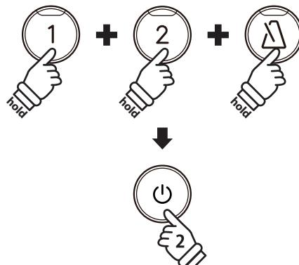
The piano will turn on in update mode, and the LED indicators for the three pressed buttons will start to flash.
