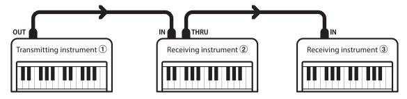
Transmitting instrument ① sends transmit channel and keyboard information to receiving instruments ②/③.
