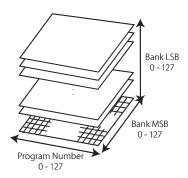
This is a 3D image of the expanded program change system with the MSB and LSB. To use these efficiently and correctly, refer to the operation manual of any external MIDI sound modules that are connected to the MP6.
