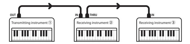
Transmitting instrument 1 sends transmit channel and keyboard information to receiving instruments 2/3.
