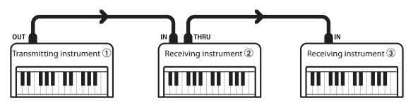
Transmitting instrument (1) sends transmit channel and keyboard information to receiving instruments (2)/(3). The information arrives at the receiving instruments (2)/(3).
