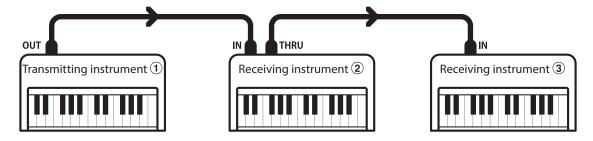
Transmitting instrument 1 sends transmit channel and keyboard information to receiving instruments 2/3. The information arrives at the receiving instruments 2/3.
