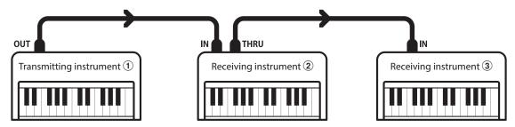
Transmitting instrument ① sends transmit channel and keyboard information to receiving instruments 2/3.
